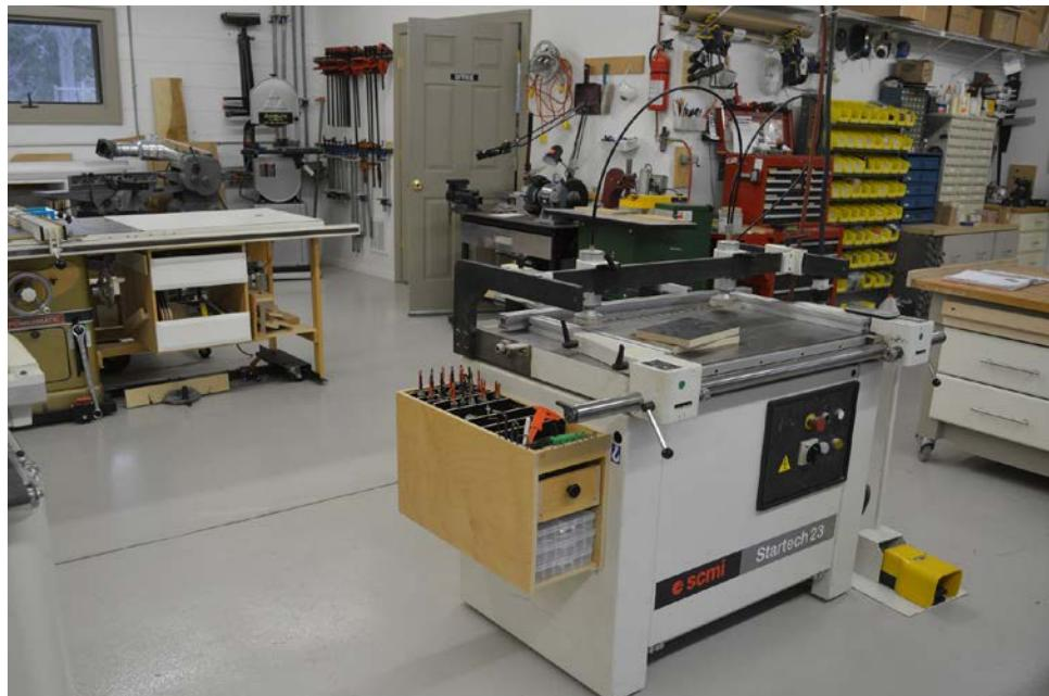
Casemarte uses all 32mm construction, so this SCMI Smartech 23 boring machine is central to the shop.
